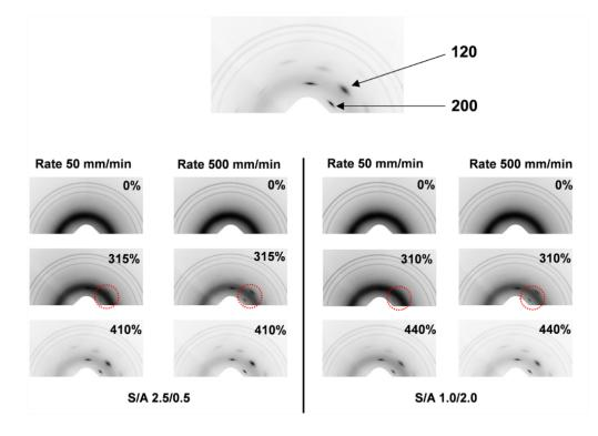
Figure 2. 2D-WAXD images of two alternative NR sample type, stretched at different rates to various strains.
