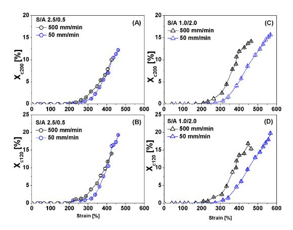
**Figure 4.** Degrees of crystallinity (Xc) for two alternative sample types at different stretching rates; (A) Xc corresponding to (200) plane of S/A 2.5/0.5, (B) Xc corresponding to (120) plane of S/A 2.5/0.5, (C) Xc corresponding to (200) plane of S/A 1.0/2.0, and (D) Xc corresponding to (120) plane of S/A 1.0/2.0.
