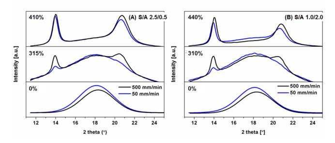
Figure 3. WAXD patterns of two alternative NR samples at different stretching rates, (A) S/A 2.5/0.5 and (B) S/A 1.0/2.0.
