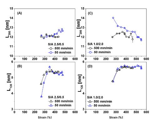
**Figure 5.** Crystalline sizes of (200) and (120) planes for sample types S/A 2.5/0.5 (A and B), and S/A 1.0/2.0 (C and D) when stretched at 50 and 500 mm/min.
