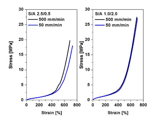
Figure 1. Stress strain curves of two alternative NR samples subjected to different stretching rates.
