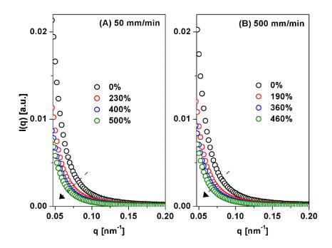
Figure 6. Representative plots of intensity versus strain for S/A 2.5/0.5 sample at the two deformation rates (A) 50 mm/min and (B) 500 mm/min.
