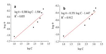
Figure 8 Freundlich adsorption isotherm of WSC from shrimp (a) and mussel (b) shells wastes.
