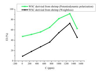
**Figure 7** The curves of WSC concentration derived from shrimp shells against inhibition efficiency by weight loss and potentiodynamic polarization methods.
