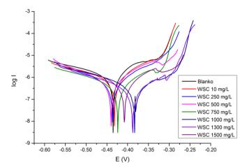
Figure 6 Tafel plots of tinplate in NaCl 2% by the addition of shrimp shells WSC.
