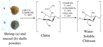
Figure 2 vvSC synthesis reaction (Du et al., 2009).
