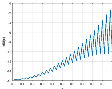
Fig. 1 Oscillation of the approximating kernel for  $m=50, \gamma=10, \xi=1, a=1$
