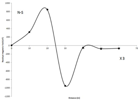
Fig. 6c Ground magnetic profile along traverse 3.
