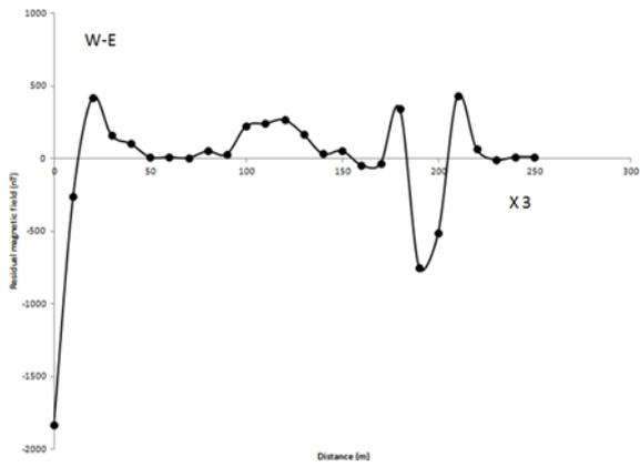
Fig. 6b Ground magnetic profile along traverse 2.
