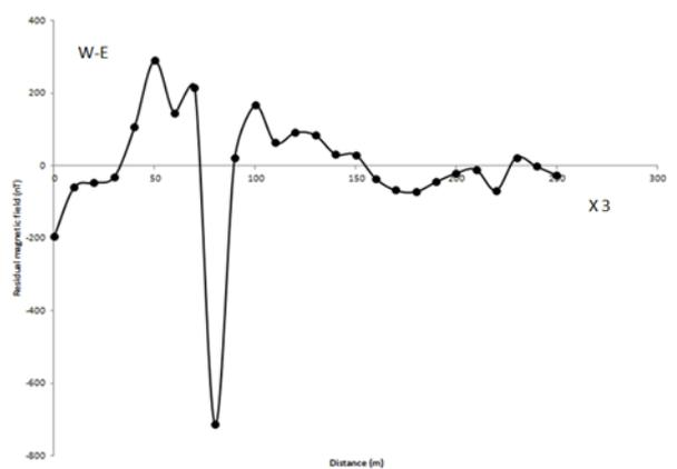
Fig. 6h Ground magnetic profile along traverse 8.
