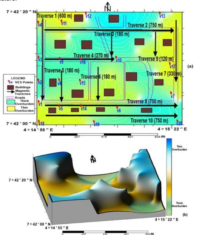
Fig. 12 (a) 2-D, and (b) 3-D: view of overburden thickness in the study area.
