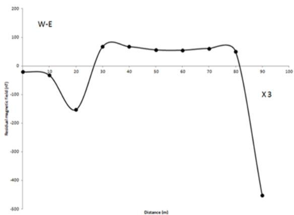
Fig. 6d Ground magnetic profile along traverse 4.
