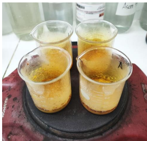
Figure 9. Preparation and digestion process of lipstick samples using aqua regia prior to Pb^{2+} analysis
