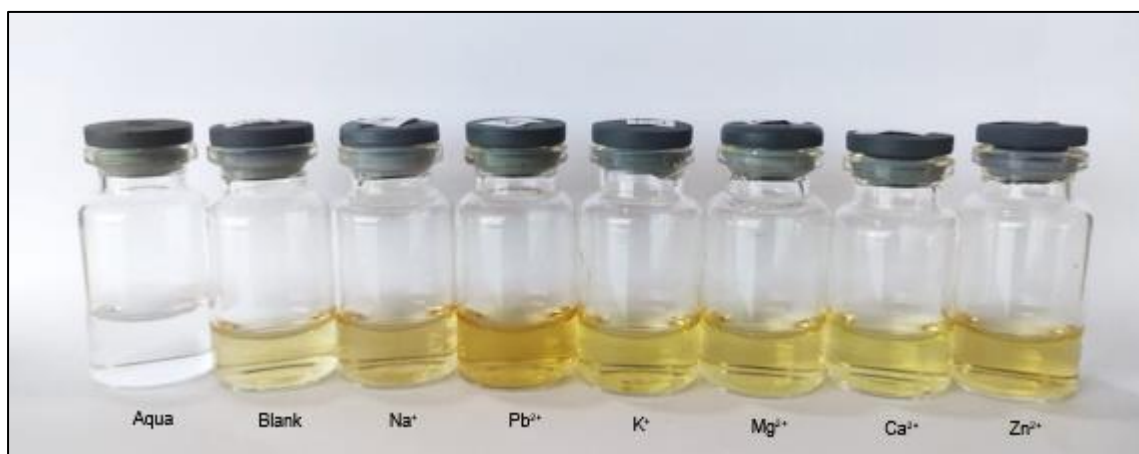
Figure 6 Visual color changes of AgNP solutions in the presence of different ions ( \text{Na}^+ , \text{Pb}^{2+} , \text{K}^+ , \text{Mg}^{2+} , \text{Ca}^{2+} , and \text{Zn}^{2+} ).
