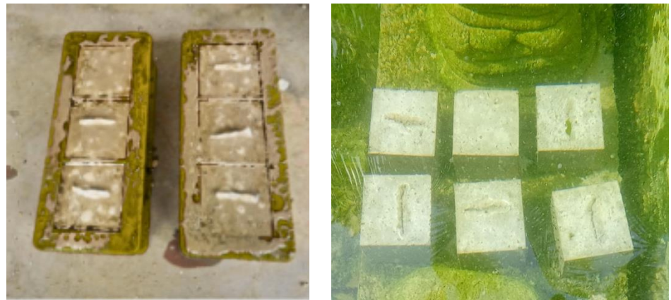
Figure 1. Mortar samples with precast crack preparation
