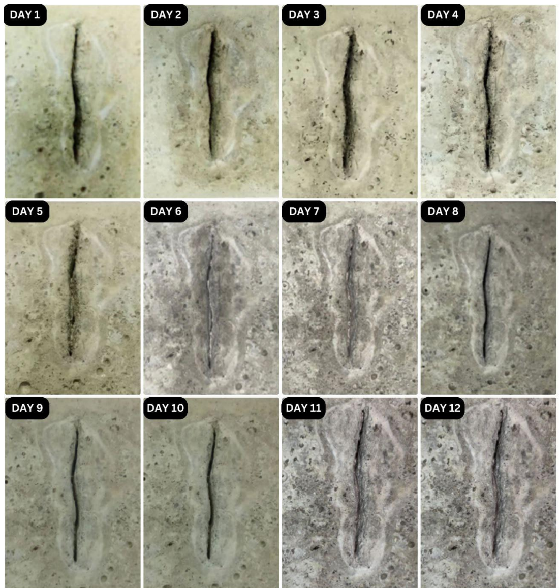
Figure 3 MICP crack repair progress using Cytophila horneckiae bacteria
