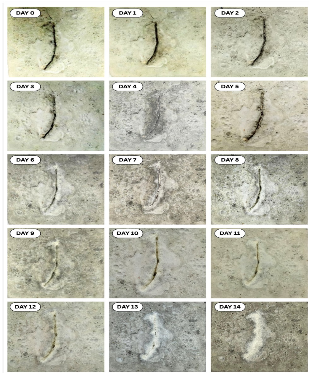
Figure 3. MICP crack repair progress using Sporocarcina Pasteurii bacteria
