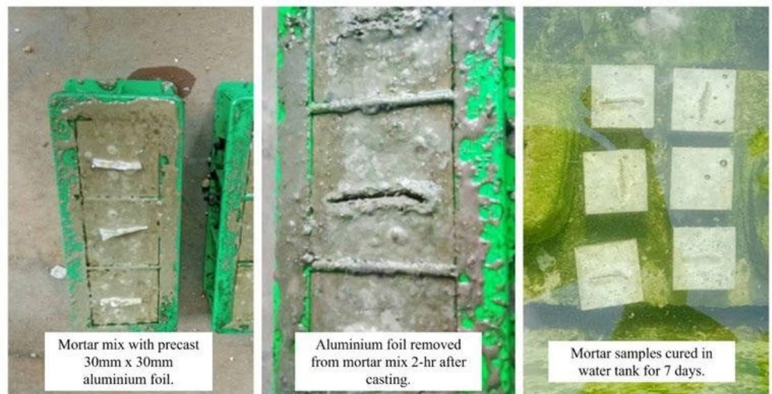
Figure 1. Mortar samples with precast crack preparation
