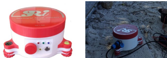
Figure 6. Seismometer SRI and measuring micro-seismic using SRI [39]
