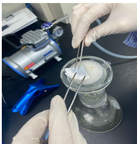
Figure 3. Folding the MCE filter membrane with the filtrate side (usually brown) in using a sterile forceps
