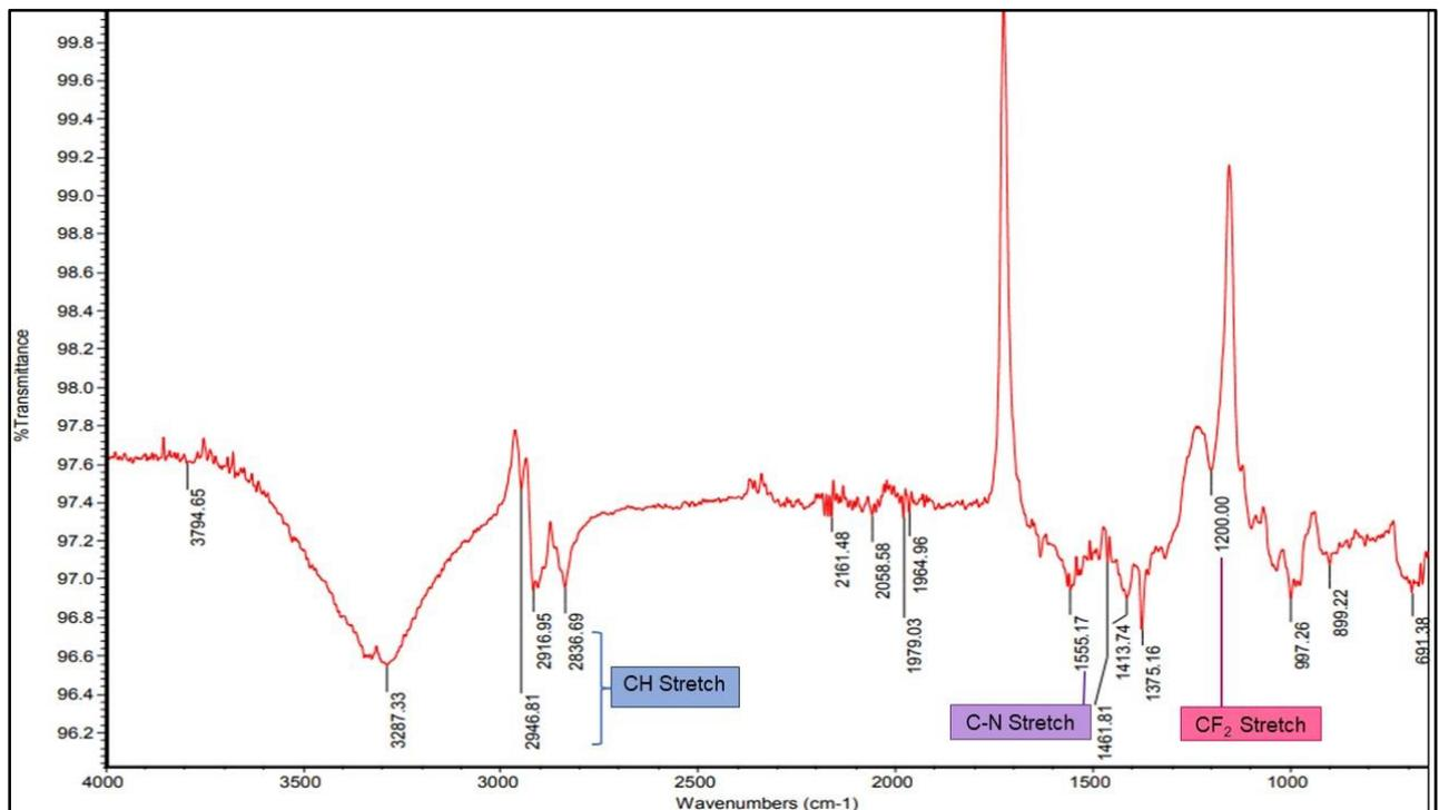
**Figure 7.** FTIR spectrum showing unidentified functional groups obtained from microplastic particles extracted from *P. undulatus* samples
