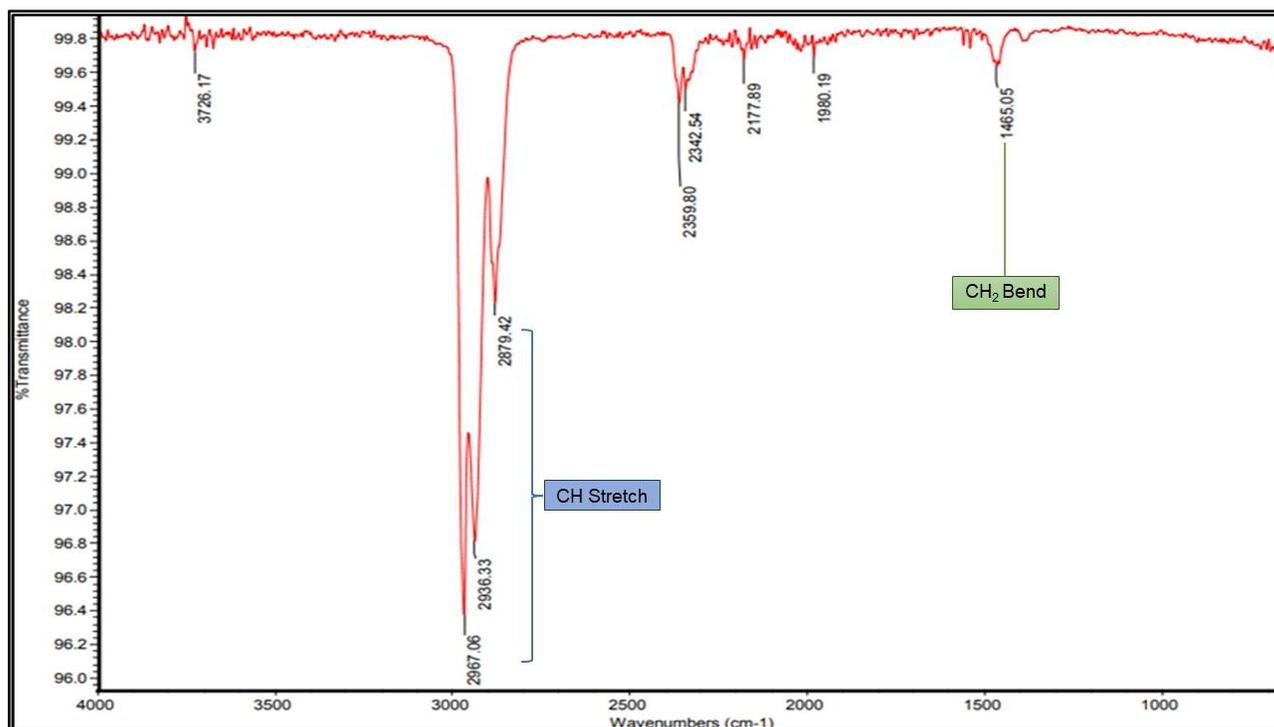
**Figure 5.** FTIR spectrum showing the functional groups of polystyrene composition obtained from microplastic particles extracted from *P. undulatus* samples
