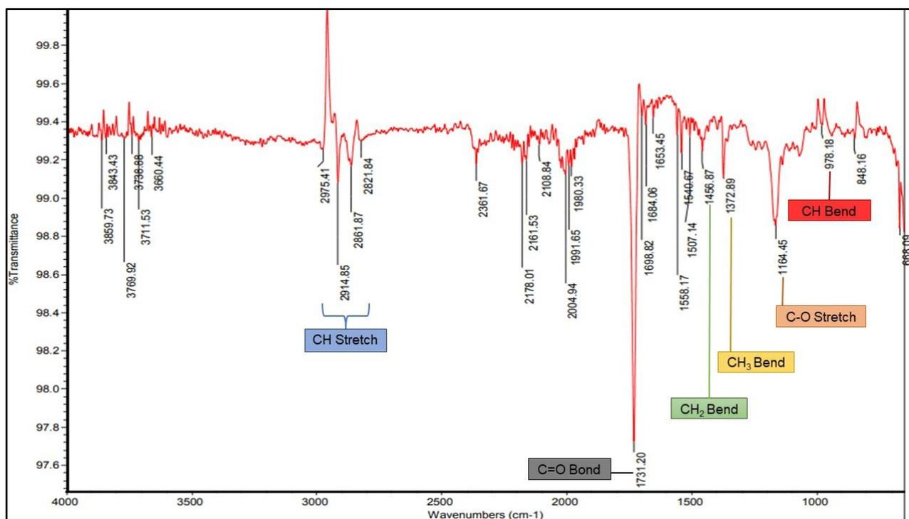
**Figure 6.** FTIR spectrum showing the functional groups of polymethyl methacrylate composition obtained from microplastic particles extracted from *P. undulatus* samples
