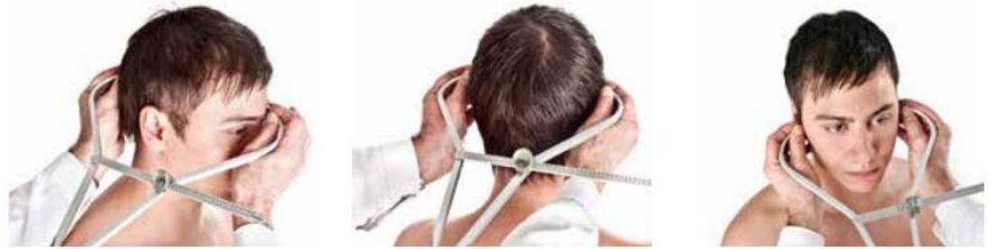
**Figure 1.** Use The Spreading Caliper To Measure Head Profile While Manual Anthropometric Measurement Process [4].
