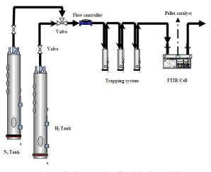
Fig. 1 : Schematic diagram of gas flow-injection technique.
