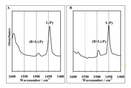
Fig. 8: IR spectra of pyridine adsorbed on Al<sub>2</sub>O<sub>3</sub> for (A) vacuum system and (B) flow system.
