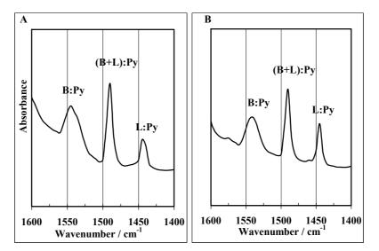
Fig. 7: IR spectra of pyridine adsorbed on Pt/SO<sub>4</sub><sup>2-</sup>-ZrO<sub>2</sub> for (A) vacuum system and (B) flow system
