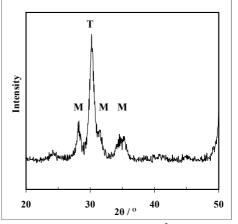
**Fig. 3 :** XRD pattern of  $Pt/SO_4^{2-}$ -ZrO<sub>2</sub>.
