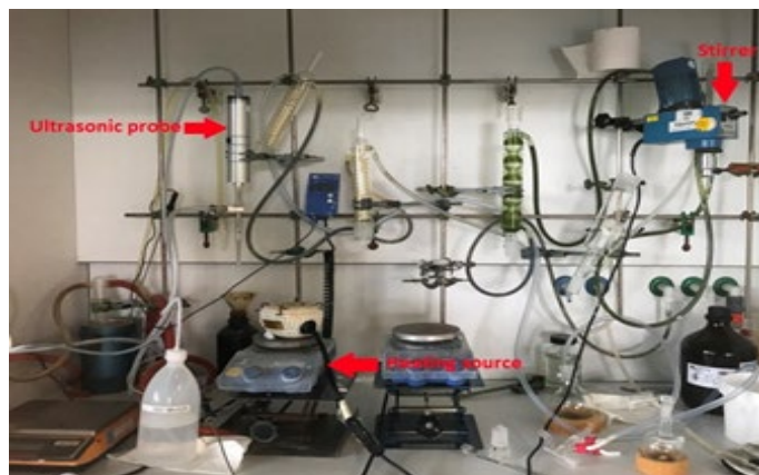
Fig. 1 Experimental setup for pre-dispersed of rGO-FT wax.
