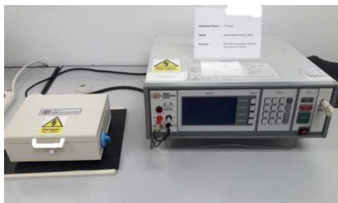
Fig. 2 Setup of Volume Resistivity Tester.
