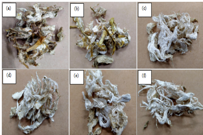
Fig. 11 Visual observation of PALF extracted at 3 % (wt.) NaOH solution concentration with cooking times of [(a) 30, (b) 60, (c) 90, (d) 120, (e) 150, and (f) 180] min.
