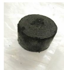
Fig. 2 Briquettes using poly(vinyl alcohol) binder with fungus growth.
