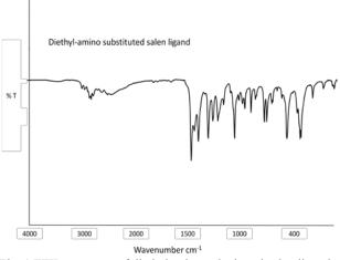
Fig. 1 FTIR spectrum of diethylamino-substituted salen ligand
