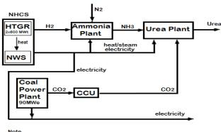
NHCS: Nuclear Hydorgen Cogeneration System HTGR: Nuclear High Temperature Reactor CCU: Carbon Capture Utilization NWS: Nuclear Water Splitting
