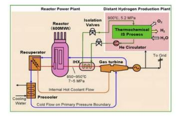
Fig. 1 HTGR for hydrogen cogeneration, thermochemical IS process [11].
