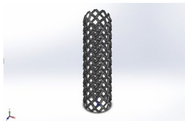
Fig. 2 Sleeve with rectangular cross section and 10 braids in number (Design A).
