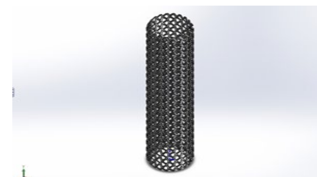
Fig. 3 Sleeve with rectangular cross section and 20 braids in number (Design B).
