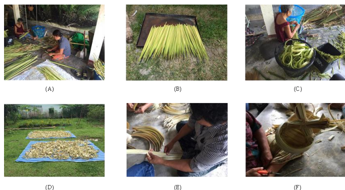
Fig. 1 The production process of Nipa bowl consists of 6 main steps: (A) cutting the top of Nipa shoots and trimming; (B) chopping Nipa shoots and sun-drying; (C) unfolding and rolling Nipa leaves in a circular motion; (D) second drying; (E) making Nipa bowls; and (F) the finished Nipa bowl.
