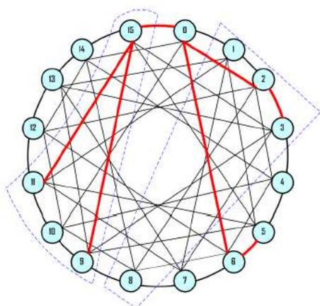
Fig. 8 CHRm6(16,1,2,4,6) Multicast Left Ring Odd and Right Chord Even Intermediate Nodes.
