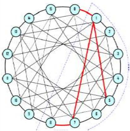
Fig. 7 CHRm6(16,1,2,4,6) Multicast Right Ring Odd Intermediate Node
