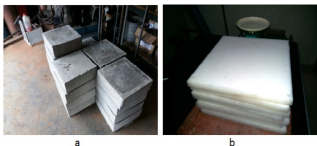
Fig.1 (a) K-500 concrete and (b) paraffin as shielding materials.
